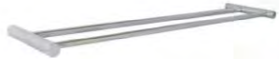
ML 6016 PSS - Double Towel Bar 620mmW ML 6018 PSS - Double Towel Bar 770mmW Mounting: (C to C) 600mm for ML 6016 PSS Mounting: (C to C) 750mm for ML 6018 PSS Overall: 145mmD Towel Bars: 12mmØ Standoff: 43mm with 63mm between
