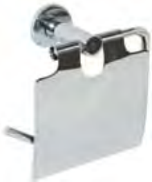
ML 6224 - Single Toilet Roll Holder with PSS Cover Overall: 145mmW x 90mmH x 85mmD Cover: 110mmW x 115mmH Holder: 7mmØ Standoff: 85mm
