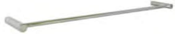
ML 6008 PSS - Single Towel Bar 620mmW ML 6012 PSS - Single Towel Bar 770mmW Mounting: (C to C) 600mm for ML 6008 PSS Mounting: (C to C) 750mm for ML 6012 PSS Overall: 95mmD Towel Bar: 12mmØ Standoff: 69mm
